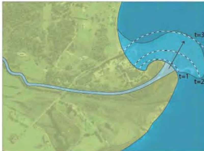
Figure 1. The progression of a deltaic lobe at the mouth of the George River and its impact on channel slope. Figure from Water Technology , 2022.
