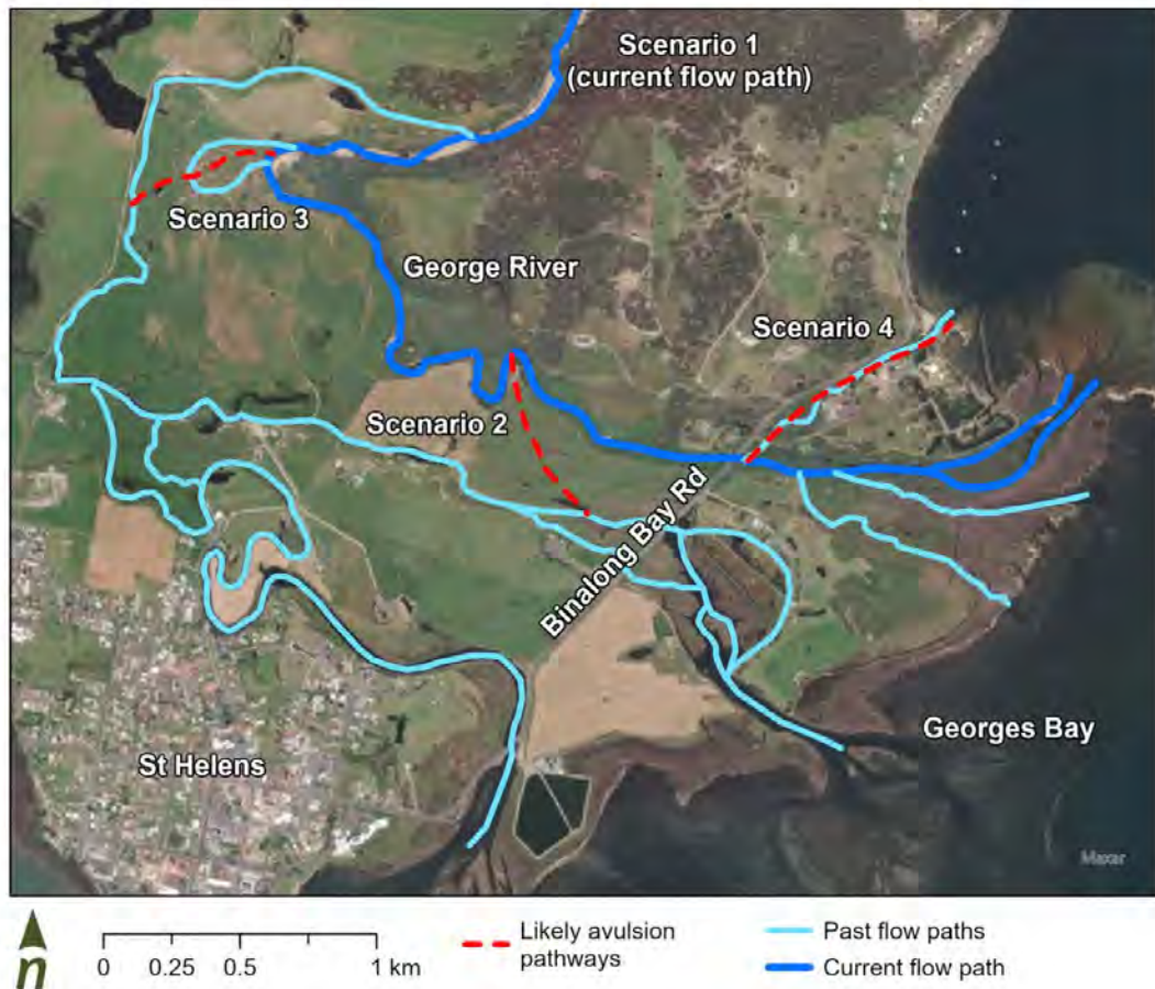
Figure 3. Overview of the four avulsion scenarios. Red dashed lines are likely alignments of newly scoured channel on the floodplain and light blue lines are channels that may be re-occupied by the George River following avulsion.
