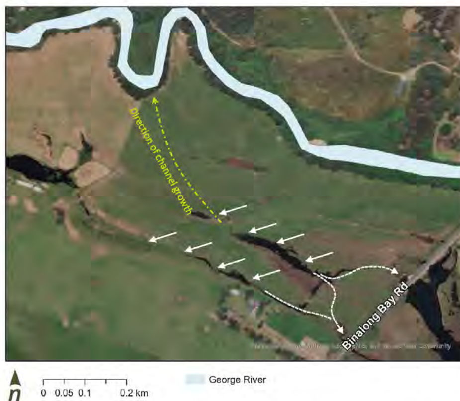
Figure 5. Scour channels that are developing on the George River floodplain. White arrows show developing scour channels, Yellow dashed arrow shows the likely direction and alignment of scour channel growth.
